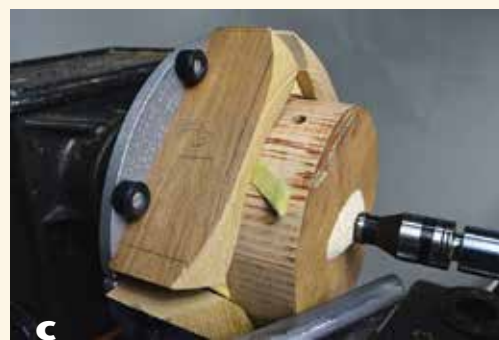
c Shims are used to adjust the position while centering the blank. The jaw's buttons visible here were used only as an aid in setting up each of the four wasteblocks, providing a reference point until the blocks were mounted with screws. The buttons are not involved in holding the wooden extensions in place. Note the protective scrap wood between the live center and the blank. The tailstock can be removed to allow access for light, final shaping cuts.
