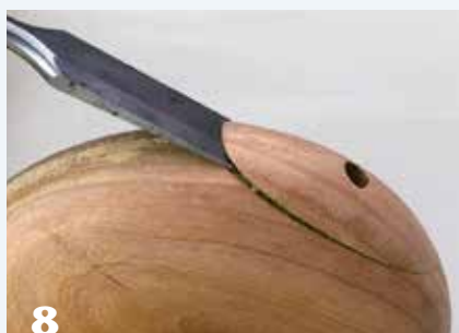
8 Use a chisel to remove the wasteblock, exposing a flat, which is critical to safe mounting on a screw chuck.
