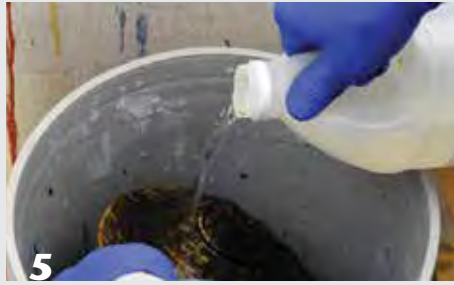
5 Rinse the workpiece with clean water to wash away excess dye from the surface. Then wipe off as much of the black dye as you can using clean paper towels. Rinse again and blot dry.
