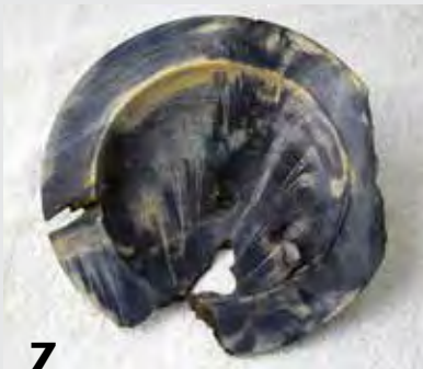
7 After the first application of dye, the piece will look blotchy. Note the difference in absorption of the black dye in varying parts of the wood, depending on grain structure.
