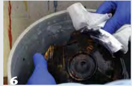
5 Rinse the workpiece with clean water to wash away excess dye from the surface. Then wipe off as much of the black dye as you can using clean paper towels. Rinse again and blot dry.
